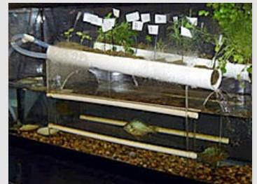
The system designed by a group of New Jersey students is an aquaponic system, which combines fish and plants in the same environment. Image Credit: Atlantic County Institute of Technology
