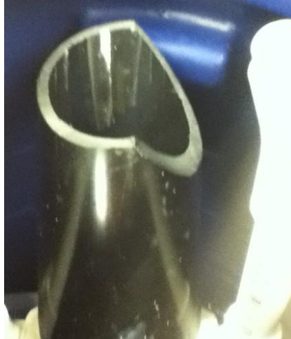
Figure 27: Tipper with side cut to maximize in flow's access to inner tipper wall
