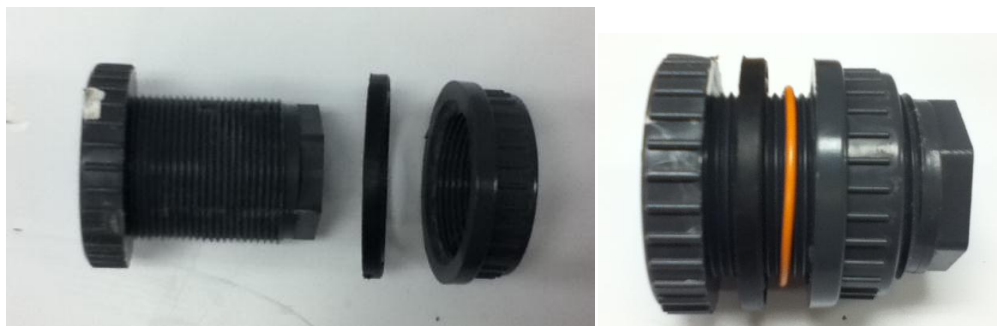
Figure 33: On the left, bulkhead Fitting exploded view. From left to right: Bulkhead screw, rubber gasket, and bulkhead threaded nut. On the right, the assembled view of bulkhead fitting. Lighter band represents the reservoir wall.
